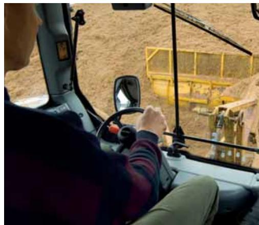
Valtra's factory-fitted TwinTrac reverse-drive system is absolutely unique in the tractor world. It is ideally suited for many kinds of agricultural, contracting and forestry tasks. The system is highly efficient and productive: Many tractor-implement combinations work best when driven in reverse, and many heavy-duty implements are always attached to the rear. The system includes a rear steering wheel with forward-reverse shuttle in the middle, plus rear clutch, accelerator and brake pedals.
