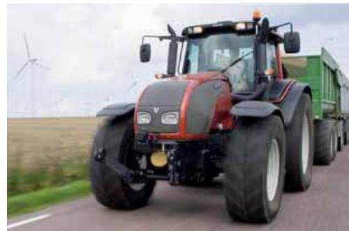
EcoSpeed is especially suitable for countries with a speed limit of 40 km/h for tractors. EcoSpeed is based on the 50-km/h transmission, but the highest speed is limited to 40 km/h. As the maximum speed is achieved in EcoSpeed tractors at a low engine speed of just 1800 rpm, and lots of driving is done at this speed, considerable advantages are created.
