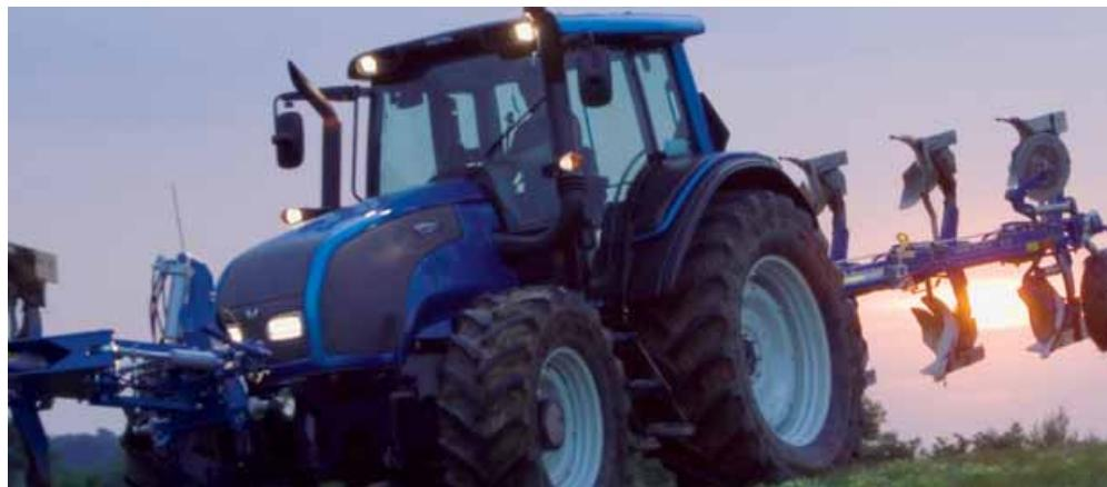
Headlands, where the tractor and implement is turned around ready for another run up the field, are areas where time can be lost while the driver spends valuable time controlling the implement and tractor. U-pilot has been developed to help the driver in these tricky situations. Valtra's U-Pilot significantly reduces the amount of repetitive work on the headland, increasing productivity while reducing fatigue. The system also reduces the risk of human error.
